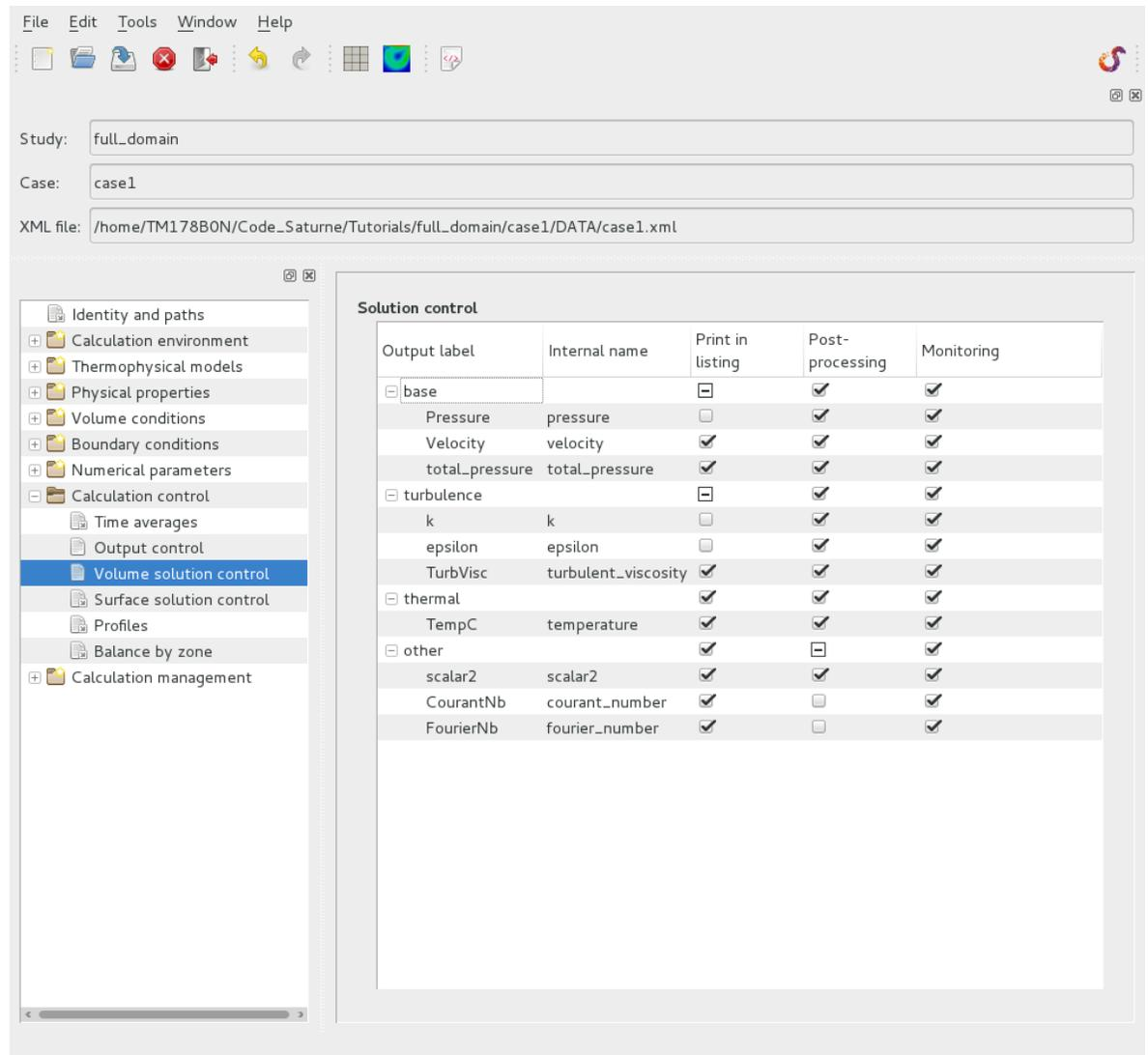
Figure III.29: Solution control: output configuration
