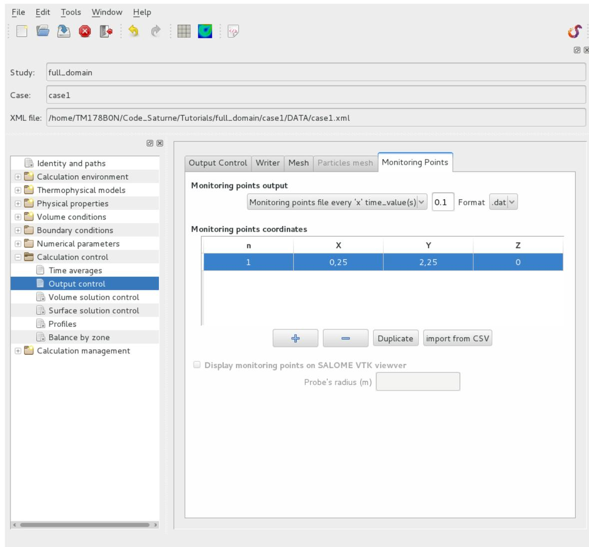
Figure III.27: Output controls: monitoring points - 1<sup>st</sup> point
