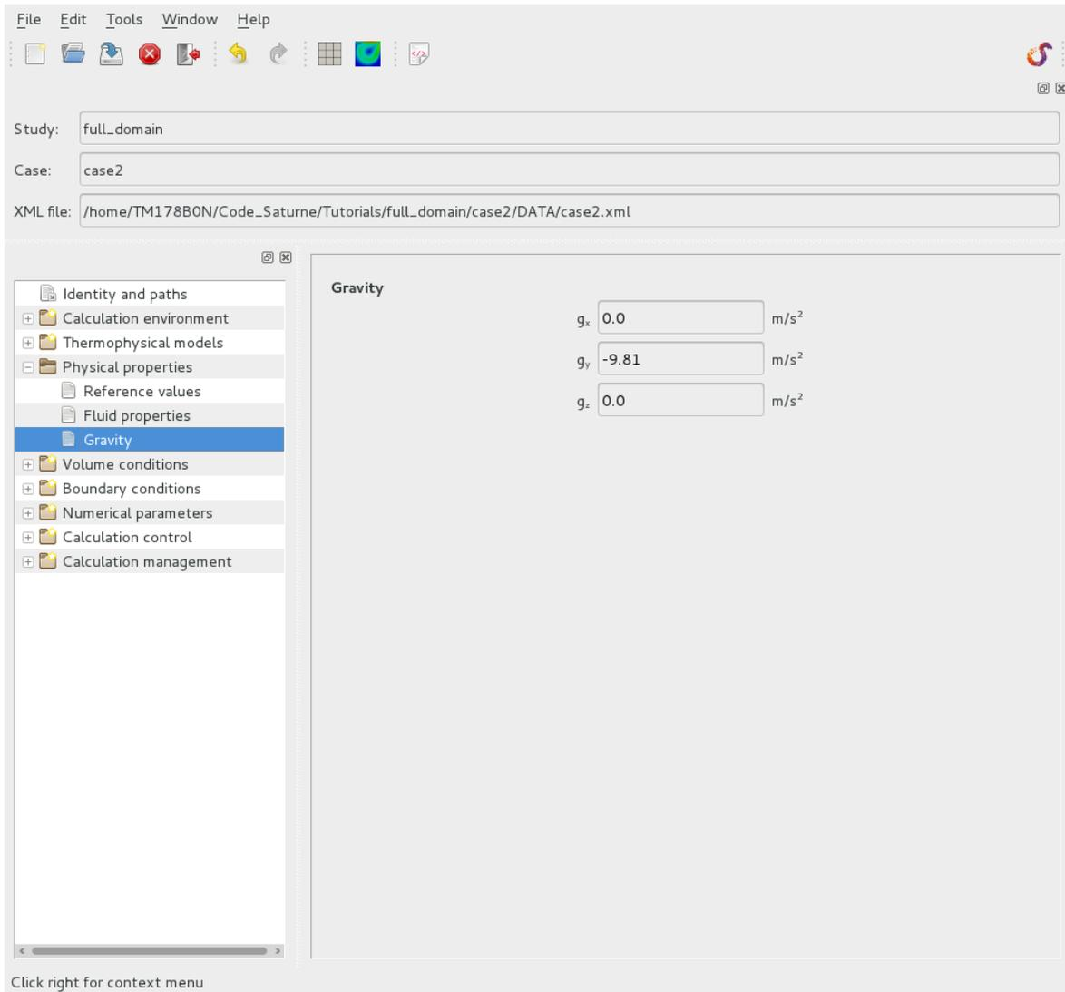
Figure III.33: Fluid properties: gravity
