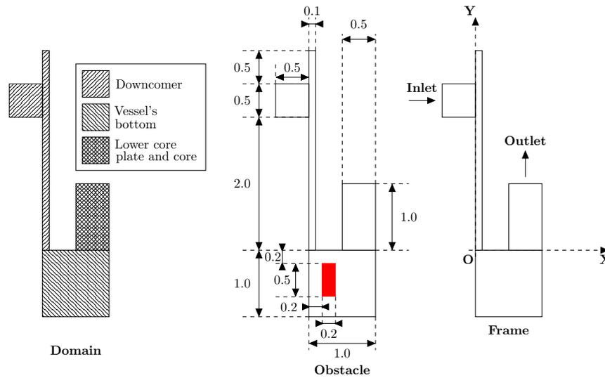
Figure II.12: Full domain geometry with the obstacle
