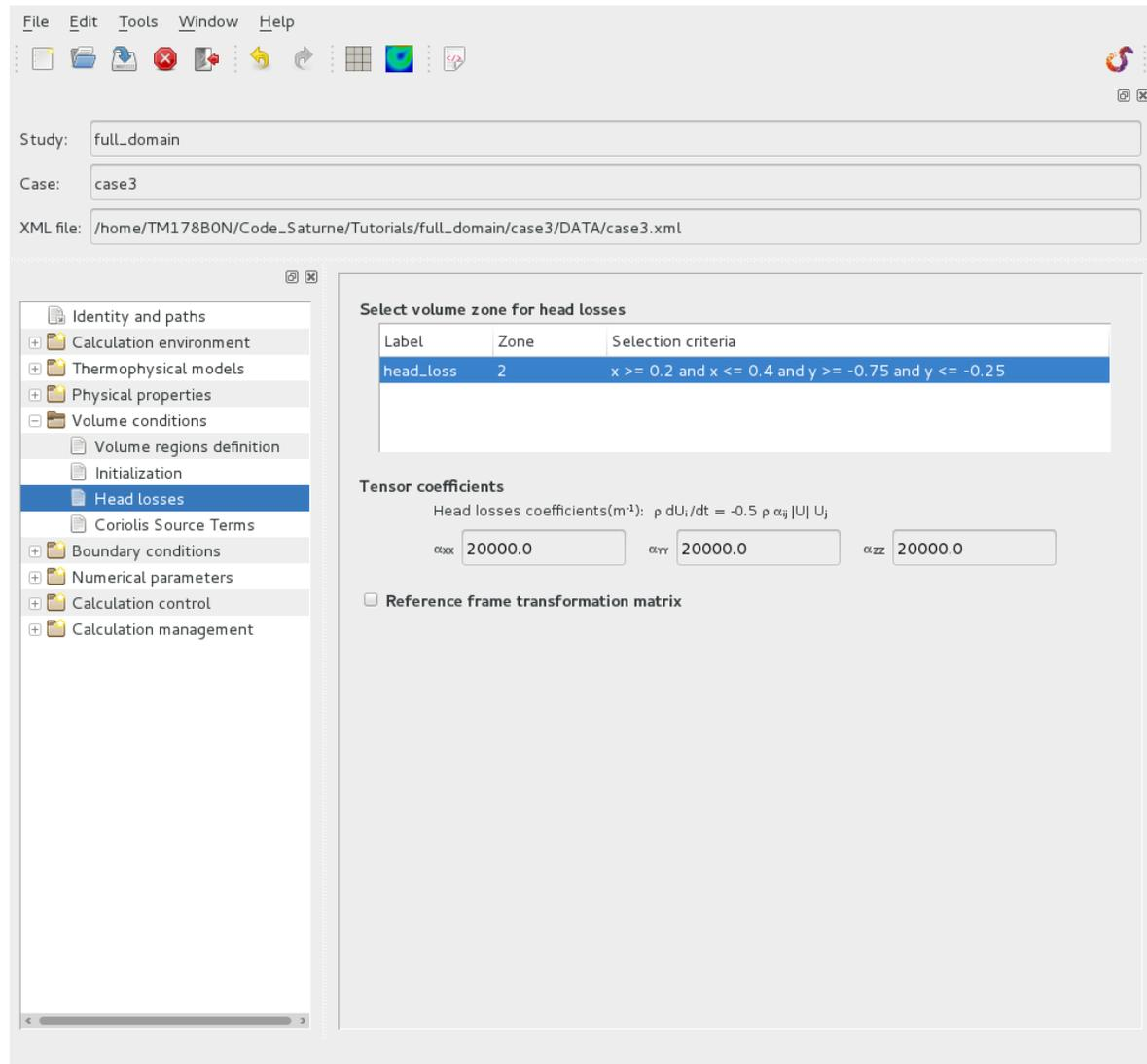
Figure III.40: Head losses coefficients
