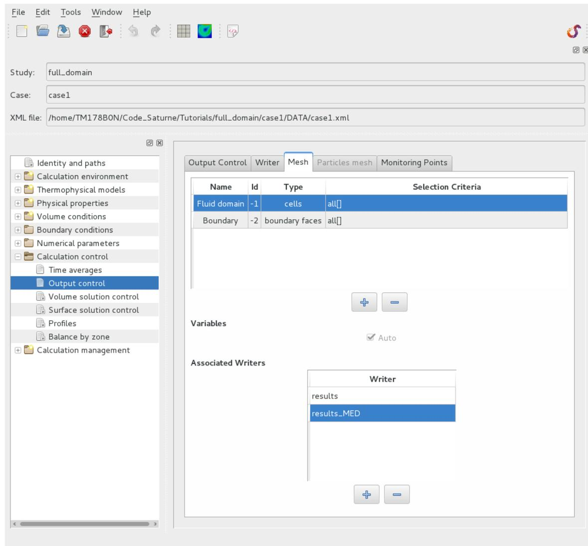
Figure III.25: Output control: associated writers
