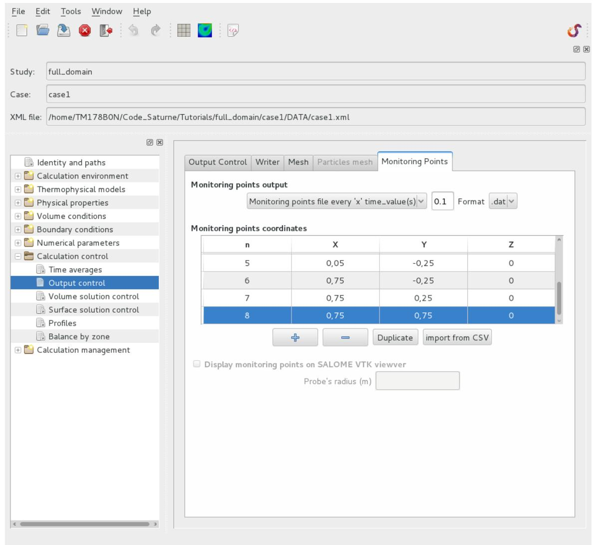
Figure III.28: Output control: monitoring points
