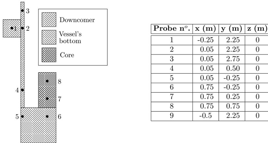
Figure II.8: Position and coordinates of probes in the full domain
