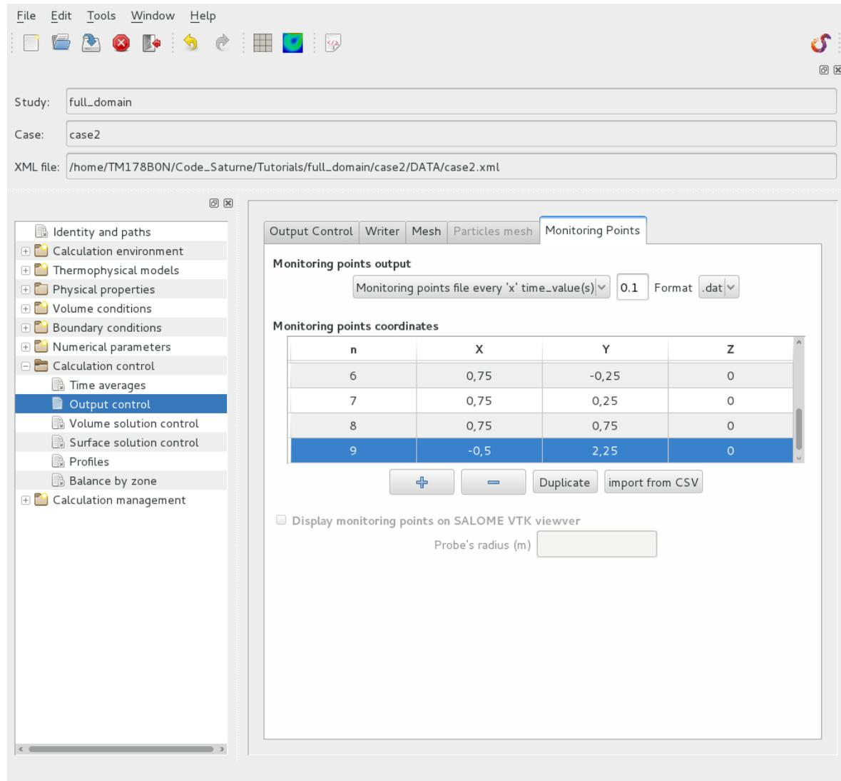
Figure III.34: New monitoring probe
