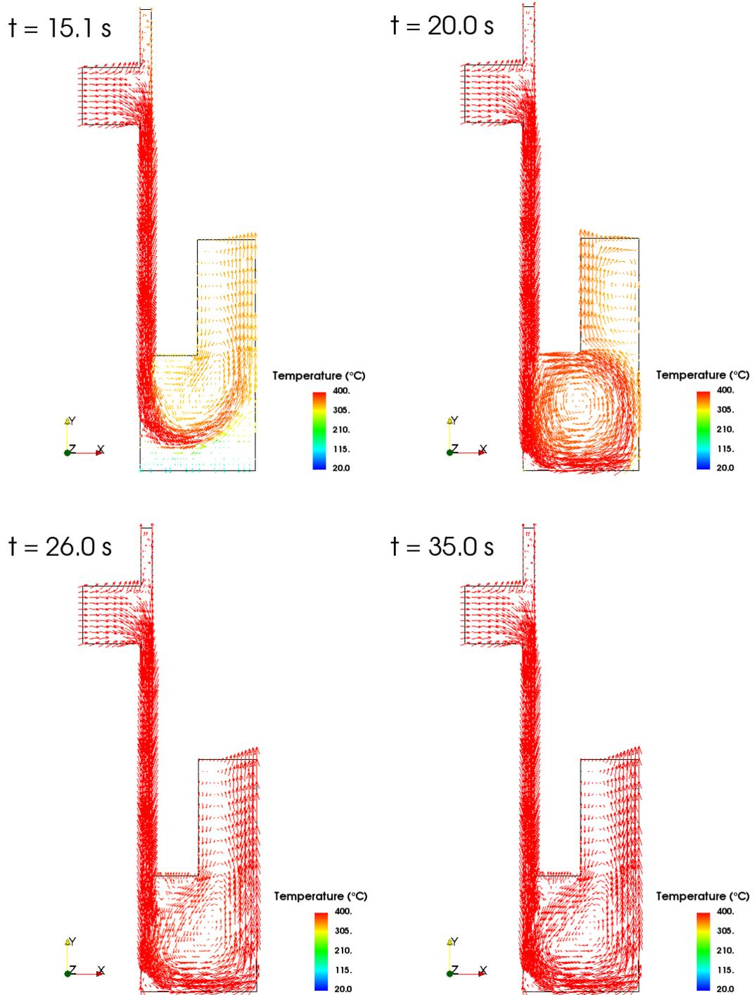
Figure II.11: Water velocity field colored by temperature at different time steps (second calculation)
