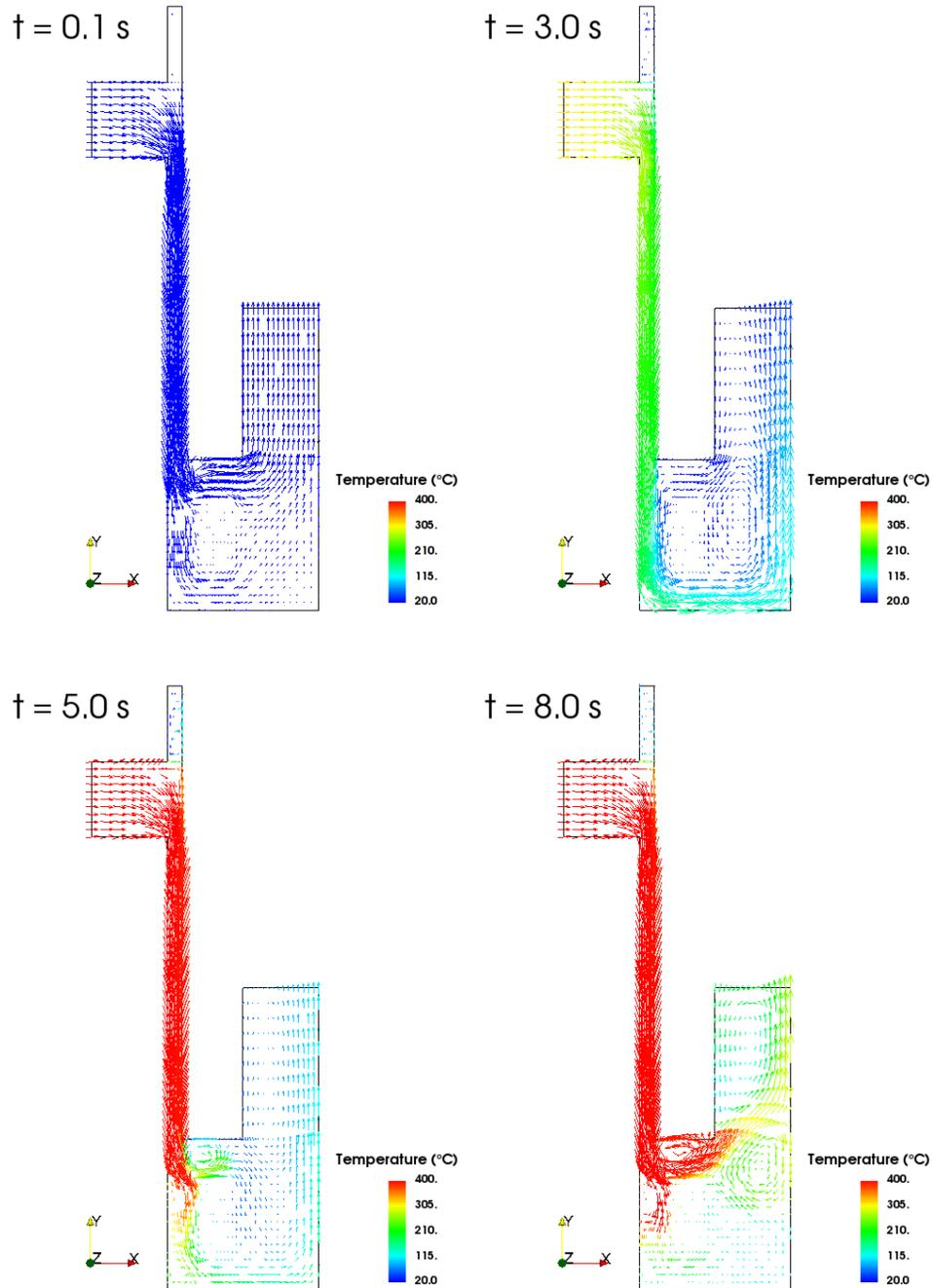
Figure II.15: Water velocity field colored by temperature - Case 3
