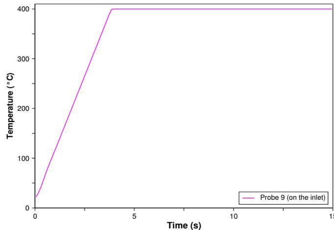
Figure II.7: Time evolution of the temperature at inlet.
