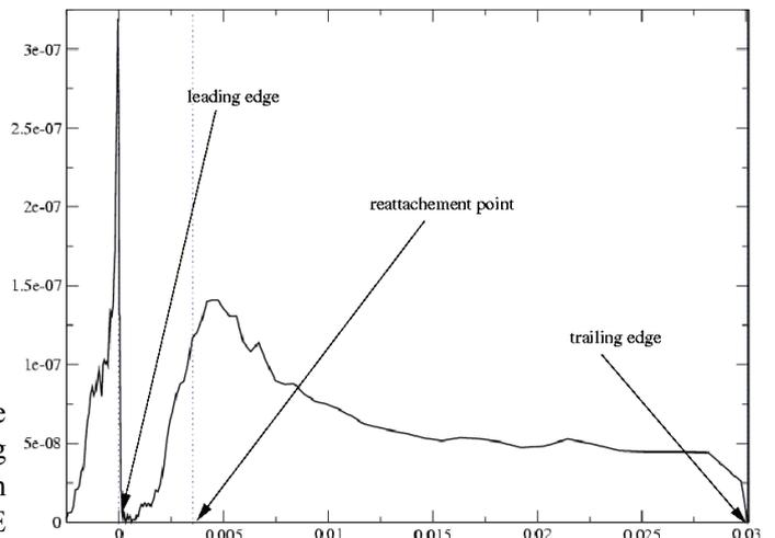
Fig. 3 : Mass flow-rate (kg/m<sup>2</sup>/s) of particles along the walls of the pipe near of the sudden contraction. The data are normalized for 1ppb of particles.
