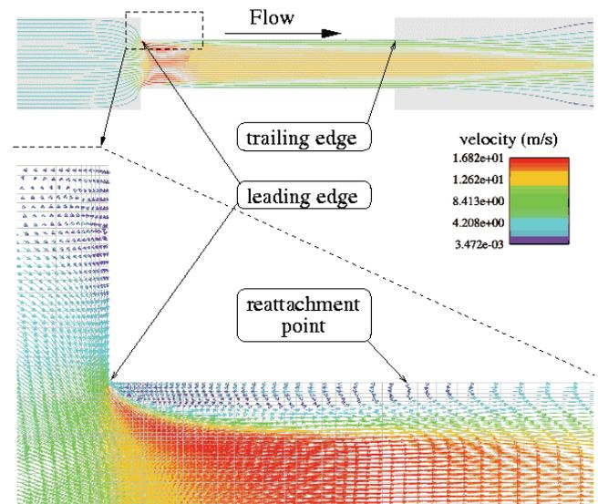
Fig. 2 : Velocity field around the sudden contraction and the streamlines. A fluid recirculation behind the leading edge can be observed.
