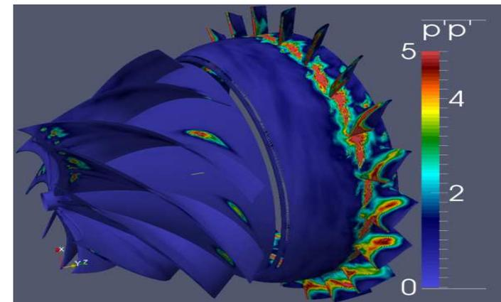
**CFD simulations of the JULIETTE 1/5th-scale PWR model for external boron dilution studies with Code\_Saturne V3.0**
