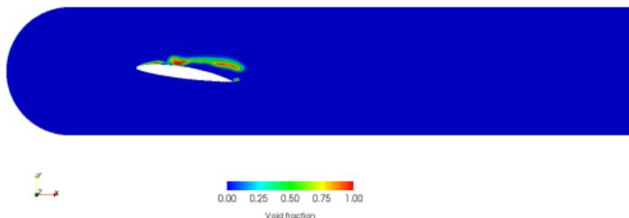
Cavitating flow around a hydrofoil
